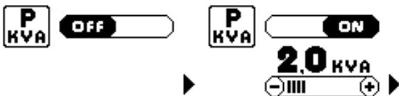
The factory default mode is OFF meaning that there is no limitation to the absorbed input power.
