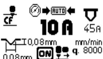
The power source automatically displays the width and depth of the groove that can be achieved with the current values (Pict. 4 Ref. G) at the relative processing speed (Pict.
