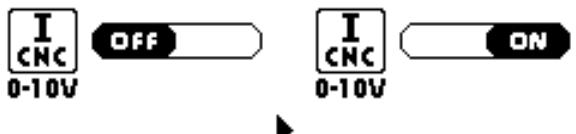
The factory default mode is OFF meaning that there is no chance of adjusting the cutting current remotely between pin 1 (0V) and pin 2 (10V).
