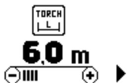
To exit the menu without making any selection, position the cursor on the arrow on the bottom right and press knob S1 (Fig.1), to confirm exiting.
