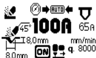
The power source automatically displays the width and depth of the groove that can be achieved with the current values (Pict. 4 Ref. G) at the relative processing speed (Pict. 4 Ref. E) set by the operator, and tells you which nozzle to use (Pict. 4 Ref. F) and the inclination in degrees that the torch needs to be maintained at during forward movement.
