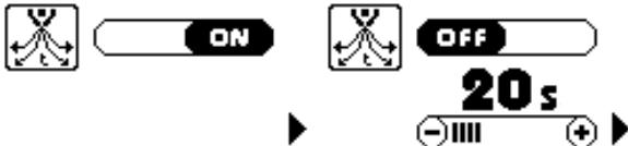
The factory default mode is AUTO ON which allows the power source to automatically and synergically adjust post gas duration based on the mounted torch, the set current value and the selected processing procedure. It is nevertheless possible to set this function on OFF so as to be able to manually adjust post gas duration (within certain pre-set limits).
